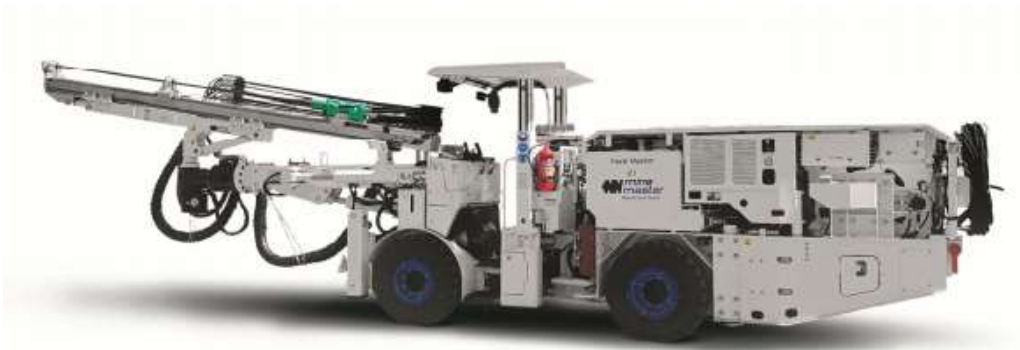
MineMaster, Face Master 2.1: Dimensionen (L-B-H): 10.2 x 1.35 x 2.1 m
