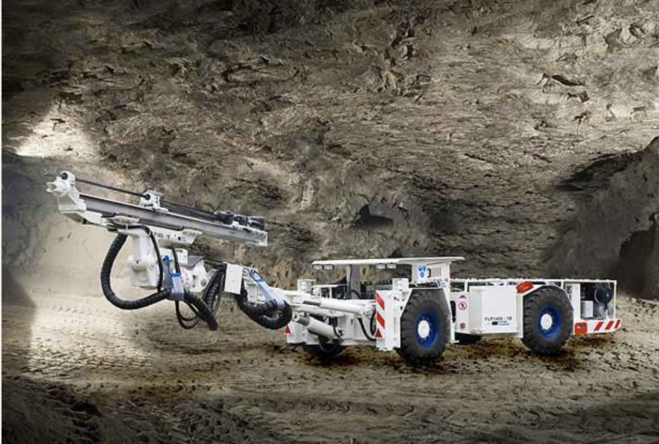
MineMaster, Face Master 2.1: Dimensionen (L-B-H): 10.2 x 1.35 x 2.1 m
